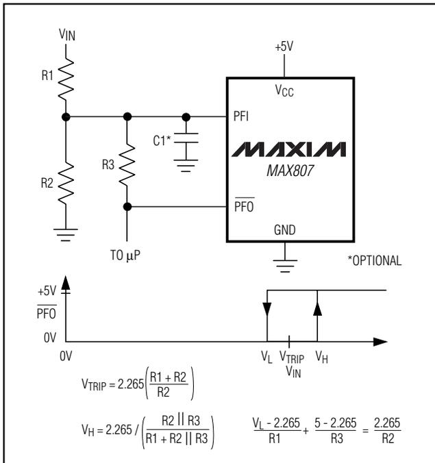
Figure 15. Adding Hysteresis to the Power-Fail Comparator
