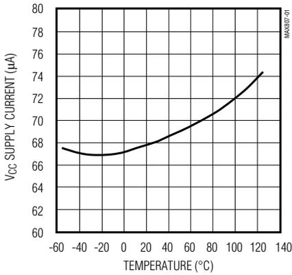
**BATTERY SUPPLY CURRENT vs. TEMPERATURE (BATTERY-BACKUP MODE)**
